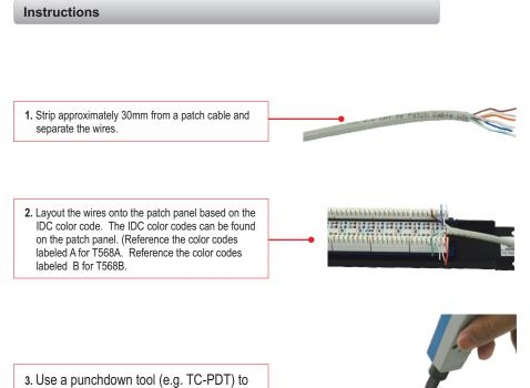
Use a punchdown tool (e.g. TC-PDT) to terminate the wires. Make sure that the cutting blade is positioned on the outside of the patch panel.
