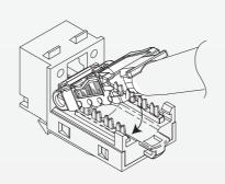
5. Feed the included cable tie through the cable fixture hole and tighten to secure the termination cap and keystone jack together.
