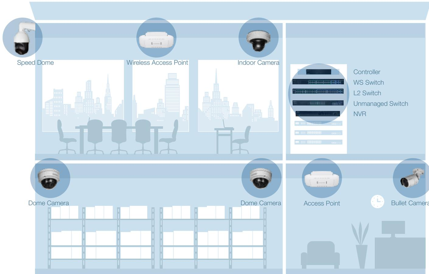
Save on setup costs and installation time by delivering power and data over a single Ethernet cable to PoE devices such as IP cameras and access points. In addition to reduced cost and time, PoE has several other benefits including flexibility for remote installations, network scalability, and managed controls. PoE delivers 15.4 watts of power per port; PoE+ delivers 30 watts; and UPoE delivers up to 60 watts of power per port.
