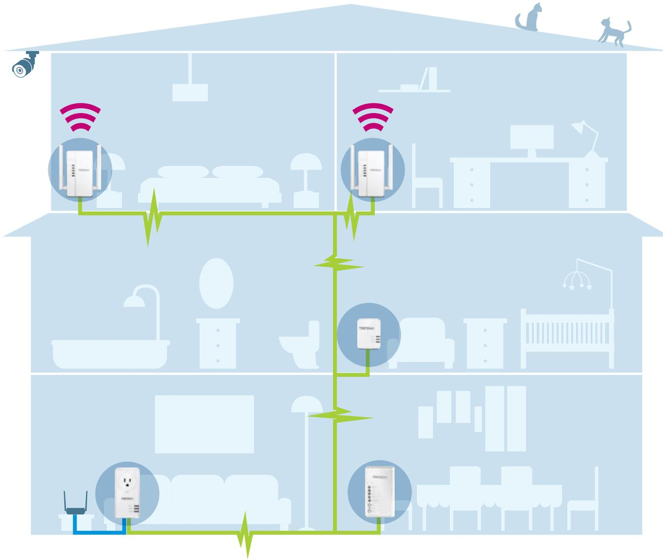
Powerline adapters can easily provide you with access to the internet from your existing power outlets. TRENDnet Powerline adapters utilize your existing electrical wiring to create or expand a wired network. TRENDnet's WiFi Everywhere™ Powerline solutions provide wireless connectivity through your power outlets with built-in access points in each adapter. These Powerline adapters are especially useful for brick and stone buildings where Wi-Fi signals have difficulty penetrating walls.
