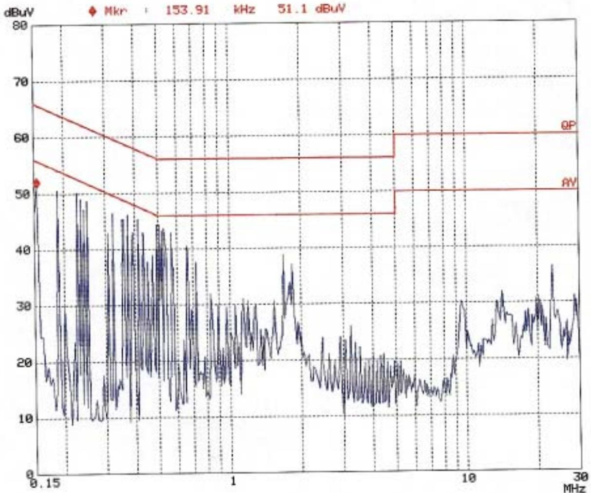
Conduction Emission Test
