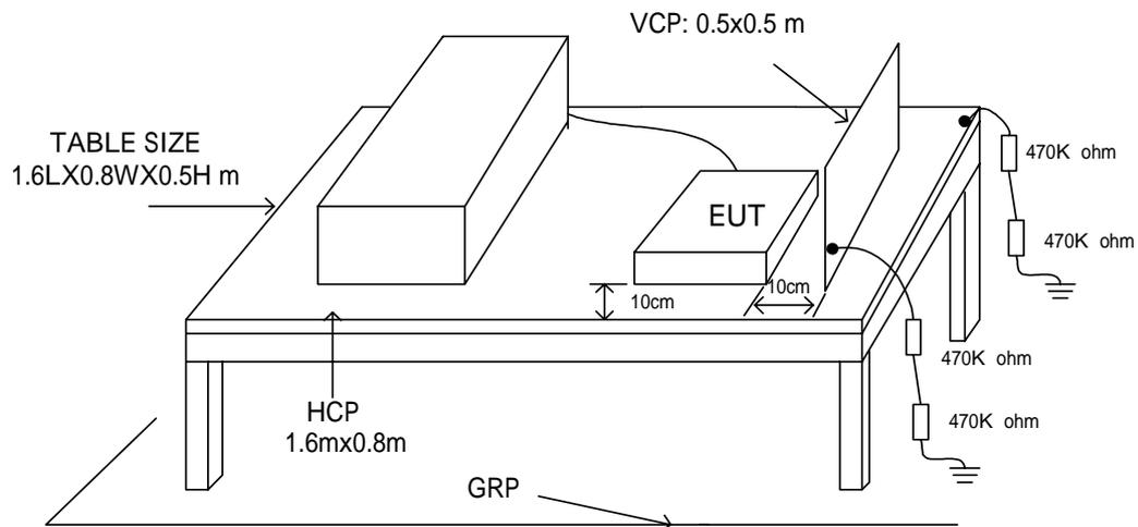
The test setup consists of the test generator, EUT and auxiliary instrumentation necessary to perform DIRECT and INDIRECT application of discharges to the EUT as applicable, in the following manner :
