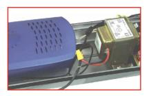
**13.** Pair the other half of the power cable with the black terminal of the enclosure's power supply.
