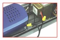
15. Take the DC plug and connect the terminals into the DC box of the camera enclosure.
