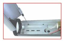
Use the following screw to mount the metal bracket onto the base of the IP Camera.
