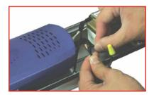
**14.** Place the yellow wire connector over the assembly in step 13, and twist the wire connector clockwise to secure the contact between the wired pair.
