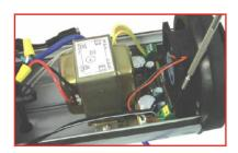
Secure the contact between the DC plug terminal and DC box by turning the screw clockwise.
